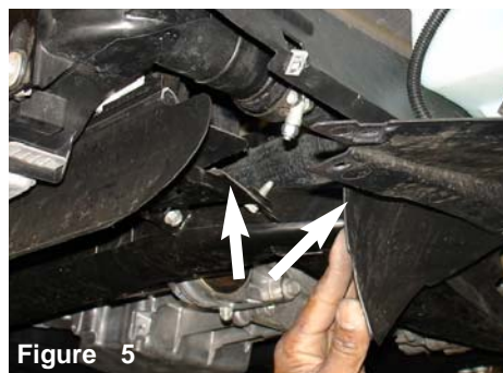
Figure 2 Driver side skid plate needs to be separated in order to expose the lower intercooler piping. a nut driver is used to remove the first m6 bolt.
