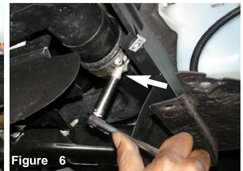
Figure 3 A nut driver is used to unscrew the second m6 bolt.
