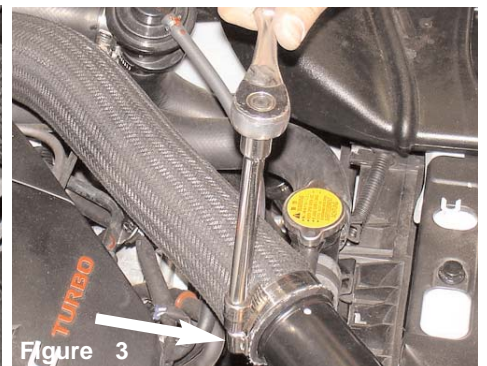
Figure 3 A nut driver is used to unscrew the second hose clamp at the intercooler outlet.
