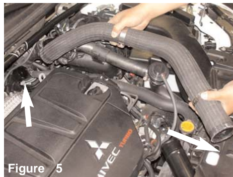
Figure 2 The upper intercooler piping hose is loosened at the turbo inlet as shown above.
