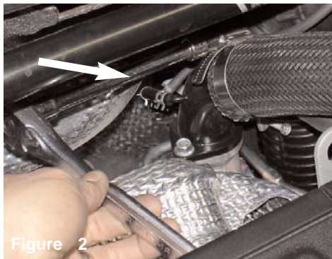
Figure 2 The upper intercooler piping hose is loosened at the turbo inlet as shown above.
